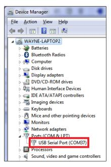
A shortcut to the device manager is provided in the File menu of RL-Loader<sup>TM</sup>. The example on the left shows a RainLog<sup>TM</sup> connected on com port 37. A new number will be assigned for each USB port on the computer. New port numbers will also be generated if you have more than one RainLog. It is suggested that you use the same USB port each time as this makes it easier to track and RL-Loader<sup>TM</sup> will automatically try the last port number used.
